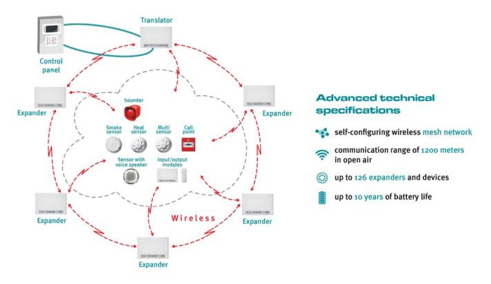
The fire alarm panel controls the alarms and events of the entire system. The wireless translator is connected directly to the wired loop of the fire alarm panel and communicates directly with the wireless devices and the wireless expanders.
